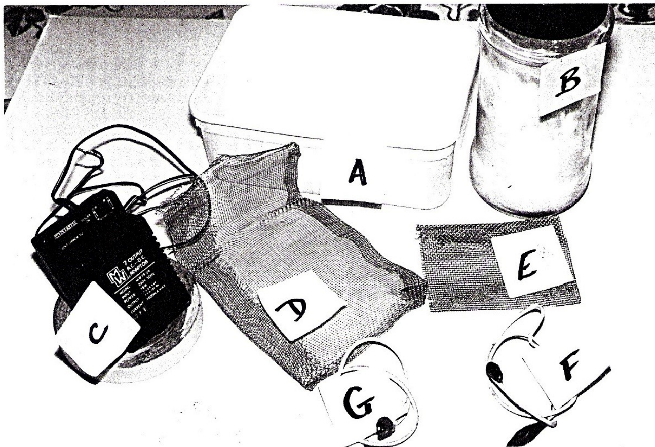
A) Ace Cream container. B) Bottle of Salt. C) Power Supply. D) Cathode mesh. E) Anode Mesh. F) Cathode fly lead. G) Anode Fly Lead
